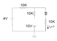
As the 10V source drives an open circuit and the  $10k\Omega$  resistor ends at an open circuit, we can neglect them. Using KVL, we can find the current through the loop using the following equation:
